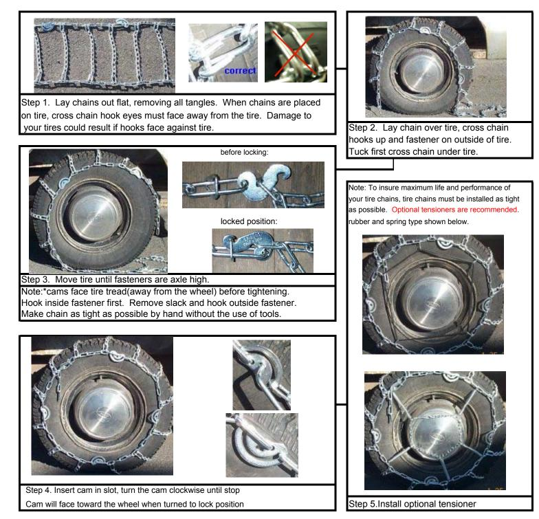
**ADJUSTMENT**: Tire chains are designed to fit a range of tire sizes and tread designs. The overall length of the chains may be longer than necessary. As long as the cross chain width is correct, the overall length can be shortened by removing 1 (or more) cross chains by prying the cross chain hook open and removing the entire cross chain. The hooks holding the cross chain to the side chain are not hardened and can be opened with a chisel or vise.
